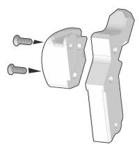
Drive 4-40 screws in through the CammerRight piece and then into the central Cammer print to create the partial Cammer assembly.
