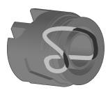
Fold an o-ring in half and push one side into the cavity in the bottom of the Base print. Then insert the other half into the other side of the cavity.
