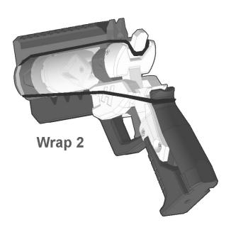
Repeat Wrap 1 with the second larger loops of elastic, but rather than lead the opposite end over the Ear of the Cammer print, leave it in the groove cut in the back of the Griddle print.
