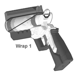
Take one of the larger loops of elastic and hook it under the hammer through the U-shaped cut at the back of the Cammer print. Wrap it up and over the Base print following the curved troughs in the front of the print.
