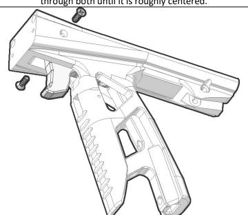
Drive a 4-40 screw into each hole to keep the short pin captive.
