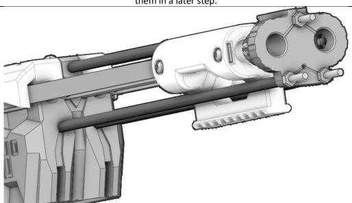
Slide the 2ndMuzzle print onto the ends of the threaded rods at the front of the assembly. Then secure it with three hex nuts.
