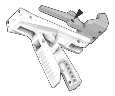
Add the aluminum sear standoff to the large hole in both Sear sub-assemblies.
