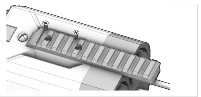
Use two 4-40 screws to attach a rail\_max print to the top of 2ndJam.
