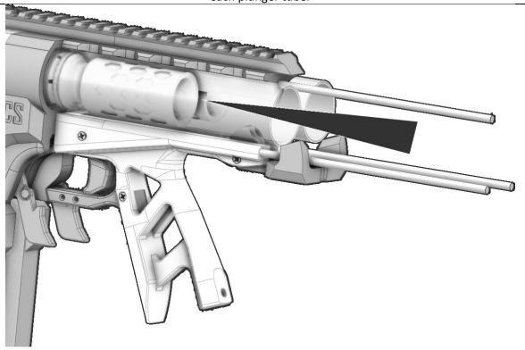
Add an o-ring to the undercut on each plunger print. Then insert one into each plunger tube.
