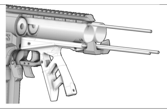
Slide the grip assembly onto the lower pair of threaded rods.
