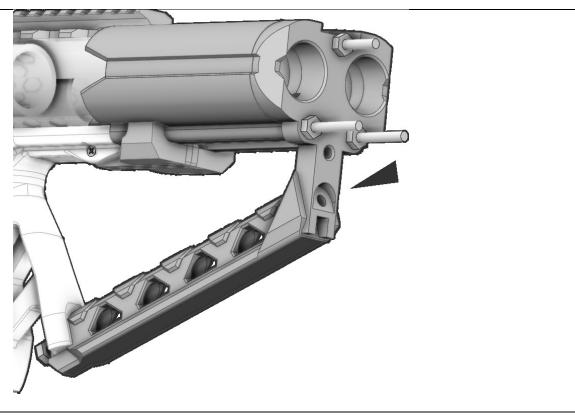
Slide an 8" length of threaded rod through the holes in all three parts. Then secure at both ends with a hex nut.
