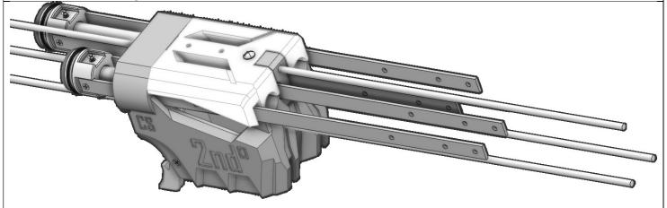
Repeat the above process for a second ramrod assembly. Then feed both into the 2ndMagLower assembly from the back.
