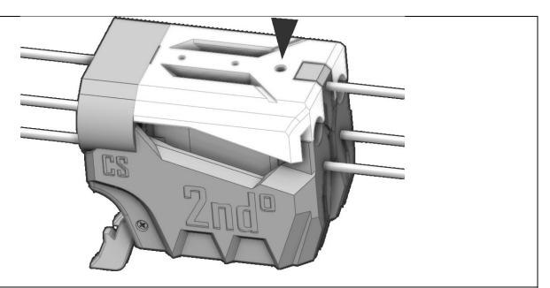
Add the 2ndJam print snugly to the top of 2ndMagLower. Use a power drill and a 3/16" drill bit to drill through both parts at this hole location.
