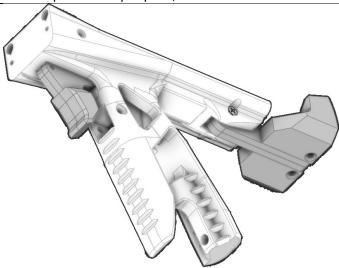
Angle both trigger half prints in through the slot in the front of the Grip5t print, then under the Sear sub-assemblies inside.
