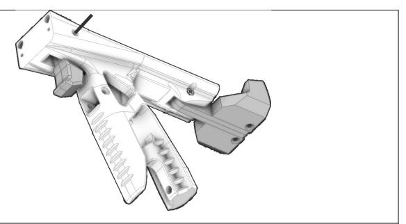
Line of the holes in all three components and push a short pin through all three.
