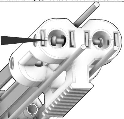
Feed a 10-32 screw into the front of the barrel hole of the 2ndForegrip print, then use a 3/16" diameter or smaller slotted screwdriver to drive it into the threaded hole in one of the central bolt arms. Repeat for the three remaining central bolt arm holes.
