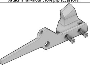
Take one of the two 2ndSearMiddle prints and attach it to the 2ndSearRight print with two 4-40 screws. Repeat to make a mirrored assembly using 2ndSearLeft.
