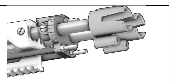
Line up the three hex nuts at the front of the threaded rods, then slide the 2ndMuzzleB onto the threaded rods until it encapsulates the hex nuts.
