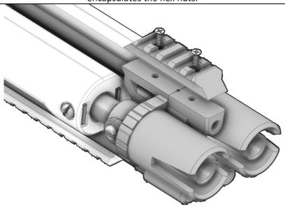
Add a rail\_short print to the top of the muzzle and secure it by driving two 4-40 screw through the holes in it.
