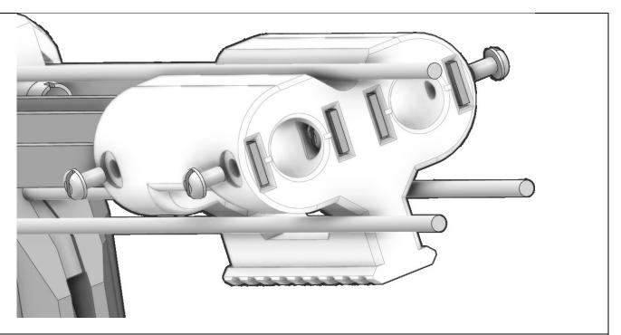
Use a short 10-32 screw to secure the outer threaded holes in the outer bolt arms.
