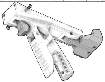
Retain the short pin by driving a 4-40 screw in from each side.
