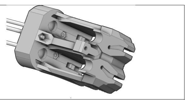
Insert a hex nut into one of the sockets inside the 2ndMagLower print. Then drive a threaded rod into it from the matching hole at the back of the print. Repeat for the other two threaded rods.
