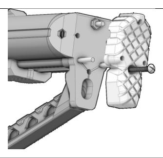
Slide the 2ndButtplate print onto all three threaded rods until it encapsulates the upper hex nut. Drive a 1-3/4" screw in through the hole in the middle of 2ndButtplate until secured.
