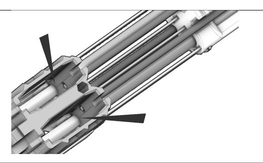
Slide a barrel into each barrel hole in the muzzle print, then into the holes at the front of the magwell. Push them in until the bottom out against the lip in the magwell, making them nearly flush with the inside of the magwell opening.
