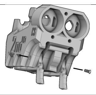
Slide a mag release print into a slot in the back of the 2ndMagLower print. Line up the hole in one of the mag release prints with the hole in the 2ndMagLower. Insert a short pin onto both. Drive a 4-40 screw into the hole to retain the pin.
