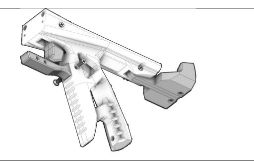
Tap it until the holes in it line up with the hole in the Grip5t print, then secure it by driving a 4-40 screw in from each side.
