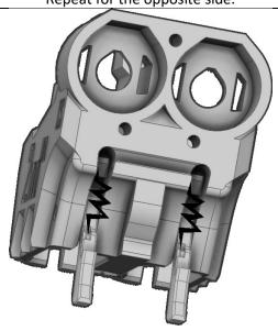
Hook the end of an extension spring onto the hook in the recessed area in the 2ndMagLower print, then onto the peg on the mag release print. Repeat for the opposite side.
