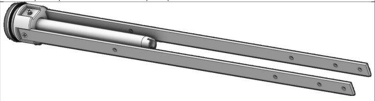
Insert a ramrod core into the ramrod base until to bottoms out against the lip in that print. Drive a 4-40 screw into the rambase print and against the ramrod core from two sides. Adhere a shock back to the back of the ramrod base print, then add an o-ring to the undercut. Use a 4-40 screw to attach the bolt arms to each side of the ramrod base.
