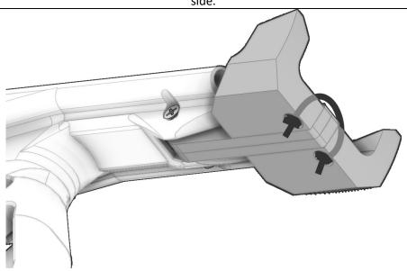
Tie a knot at the end of a short length of 3/32" diameter elastic cord. Feed it through one of the Sear halves from below, then loop over to the hole in the opposite half. Pull a little tight and tie another knot. Cut off the excess cord. The resulting loop of elastic should be as short as possible without being excessively tight.
