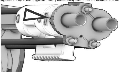
Tighten the 10-32 screws on the outside of the 2ndMuzzle print until the clamp the barrels in place.
