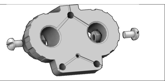
Insert a hex nut into the sockets inside the barrel holes of the 2ndMuzzle print, then drive a 10-32 screw into each one from the outer holes. Do not fully tighten these screws, as the barrel holes will need to have the barrels slide through them in a later step.
