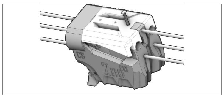
Use a slotted screwdriver to drive a 1-3/4" length screw into that hex nut through the hole in the top of 2ndJam. This will probably need to be done with both parts upside-down so that the hex nut doesn't fall out of the socket.
