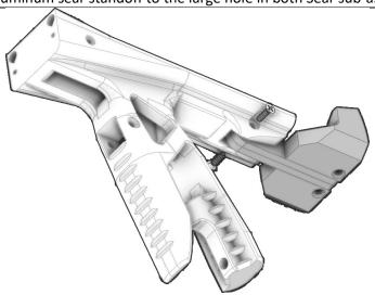
Slide it into the top of the Grip5t print, then secure it with two 4-40 screws.
