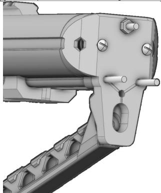
Slide the 2ndBackButt onto each threaded rod and into both main springs. Secure it with a hex nut on the upper threaded rod only.
