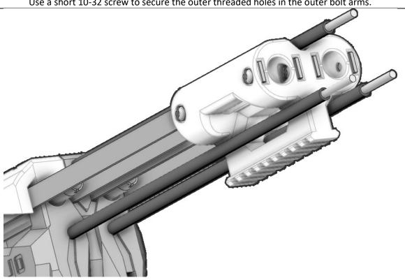
Slide a 11.25" length spacer tubing onto each of the three threaded rods.
