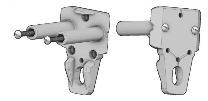
Add a hex nut to the very end of two 1-3/4" length screws, then use them to drive the hex nuts into the socket at the front of each spring guide at the front of the 2ndBackButt print. Unscrew the 1-3/4" length screws from the hex nuts. Then drive them into the back of the print and into the hex nuts from the back of the print. These screws will reinforce the spring guides and prevent them from breaking under cantilever loads.
