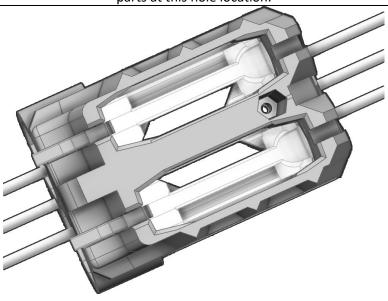
Use a slotted screwdriver to push a hex nut into the bottom of the socket from the bottom of the 2ndMagLower print.
