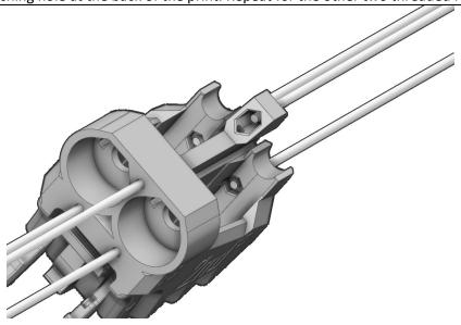
Repeat the process for all three forward threaded rods. As the build progresses, make sure that these don't protrude inside the 2ndMagLower print.
