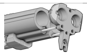
Slide the 2ndFrontButt print onto the threaded rods, and then into the 2ndStock print.
