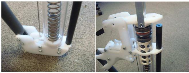
1. Seat the Plunger Tube over the pCross parts and against the stock.
