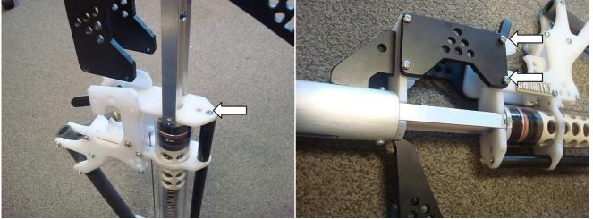
3. Insert a 3/8" length flat head screw into the hole in the top of the Mag Well Back piece, then screw it into the end of the upper stock rod.
