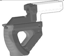
Attach a foregrip to the rail segment. Making sure that it does not extend back behind the rear surface of the rail segment. Doing so will impede priming of the blaster.
