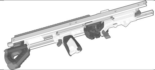
Carefully slide the remaining u-channel onto the left side of the blaster over the Triglink prints until it bottoms out againgst the whole assembly. Again, the screws that retain the nameplate may need to be loosened to allow that print to move out of the way.
