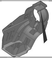
Inspect the indicated area of the Lower print for sagging filament strands. Test fit an aluminum bar inside the open rectangular slot. If obstructed by strands, use a round needle file in the indicated area to sand them down until the aluminum bar slides freely.
