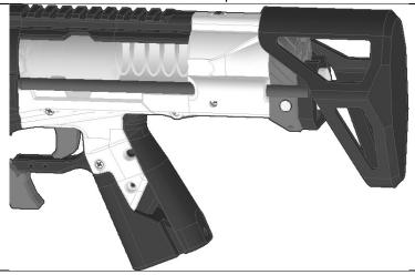
The stock can be fully collapsed, then pulled out until it locks. To adjust it (or remove it) just push up on the latch print again and slide it to a different position.
