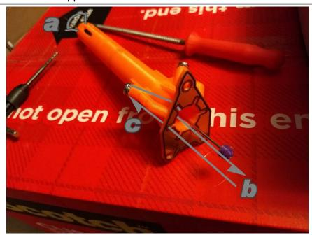
A: Remove the loose end from the Noose Wand then feed the loose end of the fishing line out the top hole at the end of the barrel, then feed it back in through the next hole in sequence.
