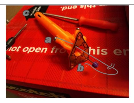
A: Take one length of fishing line and feed a loose end in through the back of one of the holes in the rear half then clamp down on it with the screw. Alternatively just tie it off around this post.
