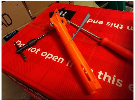
Combined the two halves of the barrel. Line up the notch in the front half of the barrel with the topmost notch of the back half of the barrel.
