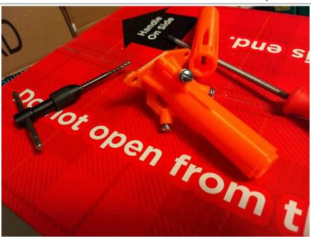
Add three 10-32 x  $\frac{1}{4}$  length screws. Do not completely tighten them. Use Scissors to cut three 24 inch long pieces of fishing line.
