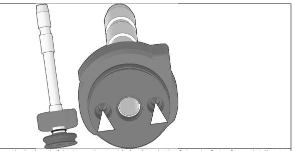
Slide the Bandle print onto the back end of the Ramrod core with the slotted side of the print facing forward. Follow it by an 012 o-ring, then the RamB print until it bottoms out against the end of the Ramrod Core.
