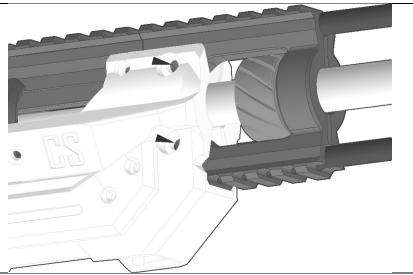
Slide the barrel assembly onto the end of the Ramrod core and the front of the magwell assembly until the holes in both lines up. Drive a 4-40 screw into each of the four holes and into the aluminum standoffs to secure the assemblies together.
