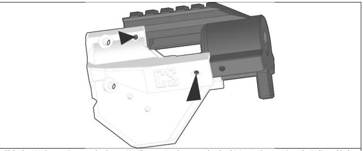
Slide the MagFront print onto the Core print. Then secure them together by driving 4-40 screws into the indicated holes on each side.
