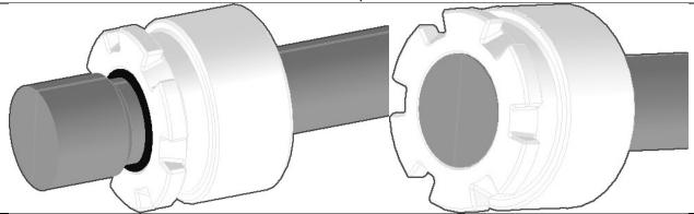
Slide the o-ring and the Phead print towards the wider end of the pair of Stem prints. Use a slotted scredriver or to push the 016 o-ring into the bore of the Phead print.
