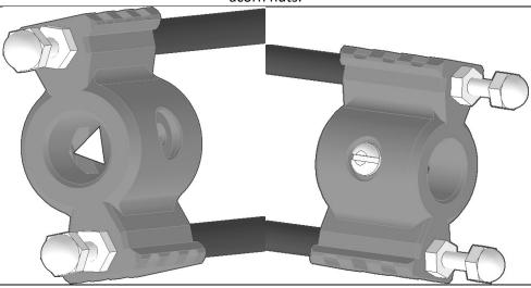
Add a hex nut to the socket on the inside of the MidBar print. Drive a short 10-32 screw into the Hex nut from the hole on the outside of the print until the end of the screw is flush with the inside surface of the hex nut.
