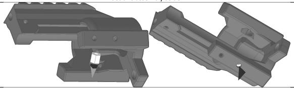
Use a slotted screwdriver to force a hex standoff into the socket on the inside of the Core print.
