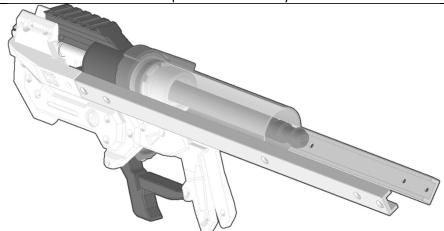
Slide the Ram assembly into the back of the Magwell. Add some silicone oil into the end of the plunger tube, then add the plunger assembly.
