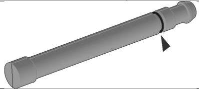
Place two Stem prints face-to-face as shown to create the Stem assembly.
