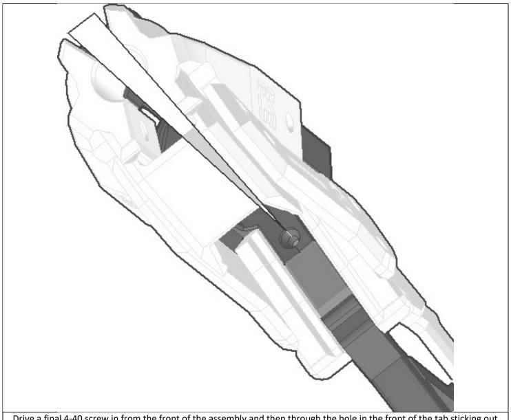
Drive a final 4-40 screw in from the front of the assembly and then through the hole in the front of the tab sticking out the bottom of the Core print.
