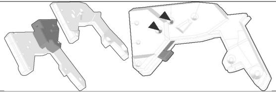
Line up the GripL and GripR prints with the holes in the sides of the MidBlock print.
