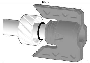
Silde the remaining Collet print, and 016 o-ring, and the Muzz print onto the exposed end of the barrel until the Muzz print bottoms out against it.
