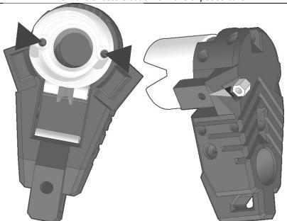
Attach the Fbutt print to the front of the Butt print using two 4-40 screws.
