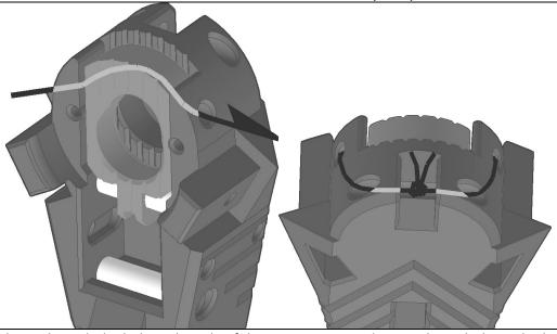
Fish some 3/32" elastic through the hole in the side of the Butt print near the top, through the arched channel inside the Sear print, then out through the opposite hole in the Butt print. Feed both free ends of the elastic into the holes further back in the top of the Butt print and out of the slot at the top rear of it.
