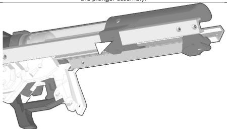
Slide the Trigger assembly in through the back of the grip. If it rubs against them too much the sides or edges of the trigger print will need to be touched up with a file.
