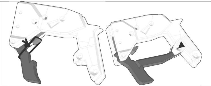
Loop some 3/32" elastic around the front of the Release print and the hook on the MidBlock print until fairly taught then tie both free ends together with a square knot. Cut the excess elastic off the tails.
