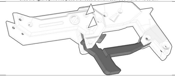
Attach the MagLeft and MagRight prints to each side of the assembly with 4-40 screws where shown.
