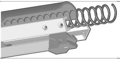
Add the main spring to the plunger tube and over the Stem of the plunger assembly.
