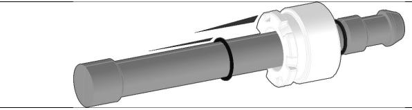
Slide an 016 size o-ring over the back end of the Stem assembly, then follow that with the Phead print. If the Phead print will not slide onto the Stem assembly then you need to go back and finish using a file to remove burrs from the edges of the Stem prints.
