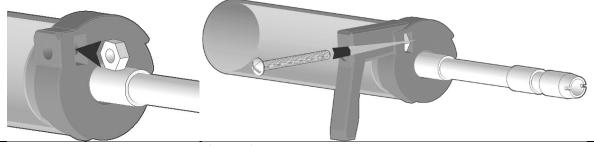
Force a hex nut into the slot in the front of the Bandle print until it lines up with the hole in the side. Line the Handle print up with the hole in both prints then feed a long 10-32 screw in through both and drive it into the hex nut until tightened.
