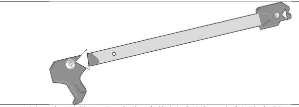
Drive a short 10-32 screw into the threaded hole in the Bolt arm that's inside the Trigger print.
