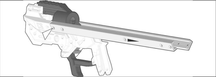
Attach a u-channel to each side of the assembly with a 4-40 screw where indicated. Make note of the center hole location on each u-channel, as they need to be closer to the back end of the blaster assembly in order for later assembly steps to work correctly.
