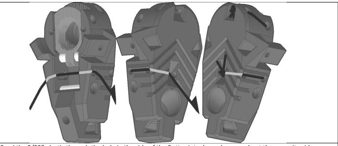
Feed the 3/32" elastic through the hole in the side of the Butt print where shown and out the opposite side. Then through the hole in the side towards the back and out through the slot at the back. Repeat for the opposite side. Pull both ends a little taught, then tie a square knot.
