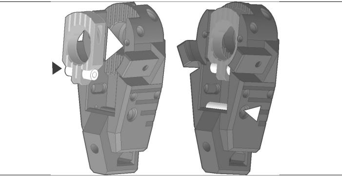
Slide a nylon spacer into the Sear print, then seat the Sear print into the Butt print. MAKE SURE THAT THE CHAMFERED SIDE of the Sear print that also has a ridged surface on it is facing forwards. Test the fit of the Sear print inside the Butt print to see if it slides freely within it. If it binds at all you will need to file or sand the sides and edges of the sear print.
