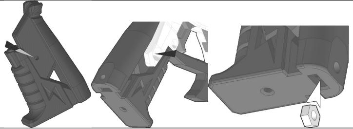
Roll a round aluminum standoff into the slot in the Griddle print until it lines up with the holes in each side.
