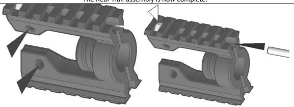
Use a ¼" drill bit or needle file to clean up the holes in the RailD print until you can force a round aluminum standoff into each one until centered.
