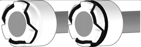
Hook a 123 size o-ring over the back of one the of the tabs on the front of the Phead print, then ahead of the next, then behind the next, and so on until it wraps around them like so.
