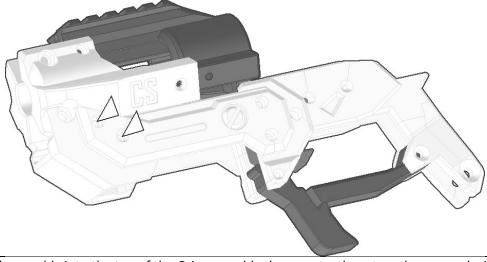
Slide the Magwell assembly into the top of the Grip assembly then secure them together on each side using two 4-40 screws where indicated.
