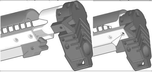
Slide the Butt assembly over the main spring and into the U-channel pair until it bottoms out. Secure it from each side by driving a 4-40 screw into the retained hex standoffs.
