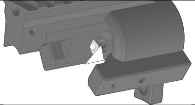
Drive a 4-40 screw into the angled hole next to the hex standoff on the inside of the Core print until the head of the screw bottoms out against the hex standoff.
