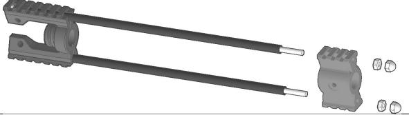
Slide the 11-1/4 long spacer tubing (or three Rail prints) over the threaded rods and into the RailD print until they bottom out.
