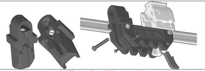
Use a screwdriver or the outside of a 3/8" socket to force a 10-32 hex nut into the hex socket inside the barrel hole in the MagFront print.
