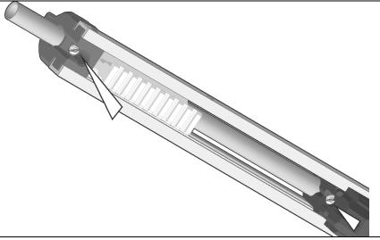
Tighten both screws indicated to clamp the barrel in place.
