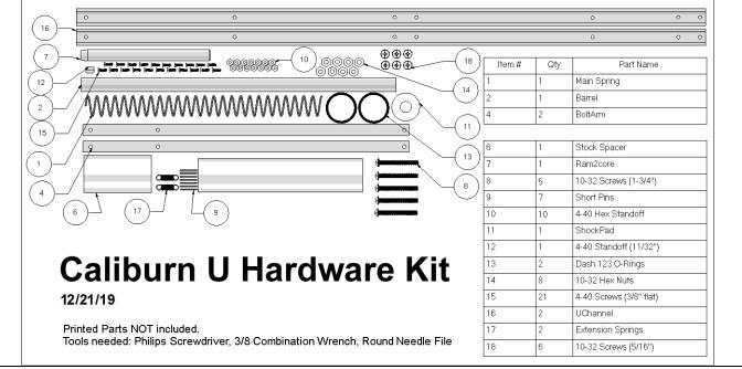
For most of the above hardware list the quantities are the MINIMUM required for assembly. Easily-lost items will have several spares and I typically include extras of the majority of the items.
