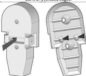
Use a slotted screwdriver to insert a 4-40 hex standoffs in through the middle of the Buttplate print until it bottoms out in the socket. Repeat on the opposite side. Drive some 4-40 screws into the holes perpendicular to the standoffs to retain them.
