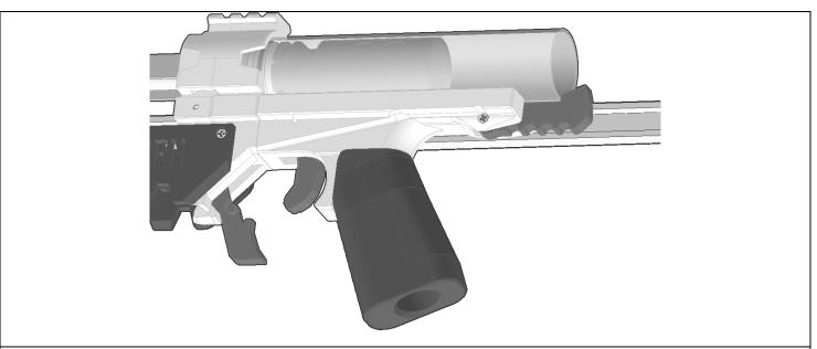
Force the Grip Assembly into the U-Channel and up against the back of the Magwell assembly.
