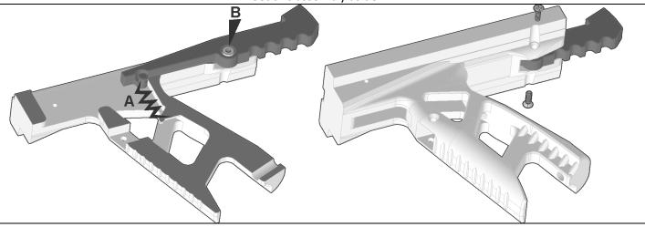
Add an extension spring to the peg on the Sear5 print, then use the print to fish the opposite end of the spring into and through the Grip print. Use an awl or a small flat screwdriver to pull the loop of the extension spring onto the hook inside the Grip5ar print.
