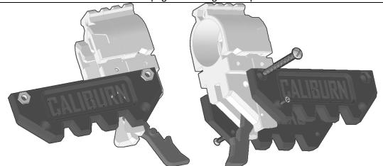
Insert a hex nut into each of the sockets in one of the nameplate prints using a hammer. Line up both NamePlate prints with the hole in the side of the Magback print and secure it with a long 10-32 screw. Drive 4-40 screws in through the lower holes to help retain the magrelease pin. Do not overtighten these screws.
