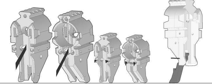
Force a hex standoff into each of the four sockets in the MagBack print. Drive a 4-40 screw into each hole indicated until they bottom out.
