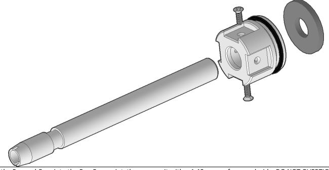
Push the Ramrod Core into the RamBase print, then secure it with a 4-40 screws from each side. DO NOT OVERTIGHTEN. Add an o-ring to the undercut in the RamBase print, then add the adhesive-backed Shockpad to the back face of the RamBase print.
