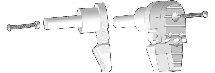
Place a 10-32 hex nut onto the end of a 1-3/4" length screw, then push the hex nut into the front of the spring guide of BackButt until it bottoms out. Unscrew the long screw from the hex nut.
