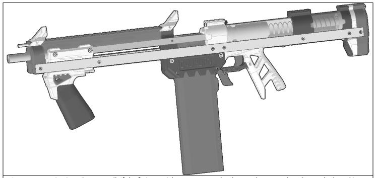
Insert a magazine into the magwell. If the fit is too tight you may need to loosen the screw that clamps the barrel into the muzzle, then the two that attach the front of the NamePlate prints to the MagFront print. Then retighten once the magazine fit feels correct.
