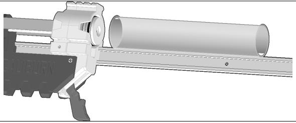
Slide a Plunger Tube over the Ramrod base and into the back of the PCap print.
