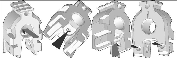
Use a screwdriver or the outside of a 3/8" socket to force a 10-32 hex nut into the hex socket inside the barrel hole in the Muzzle print.
