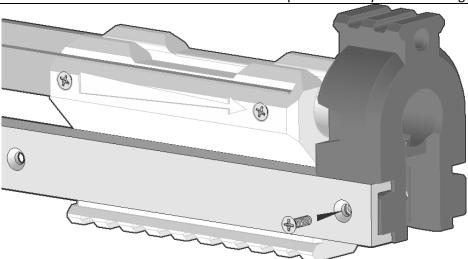
Attach the Muzzle print to the front end of the U-channel with a 4-40 screw.
