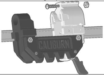
Slide a magazine into the open magwell to check fit. If the fit is too tight loosen then retighten the upper pair of long screws. Once fit of the magazine is confirmed, tighten the lower 4-40 screws the rest of the way.
