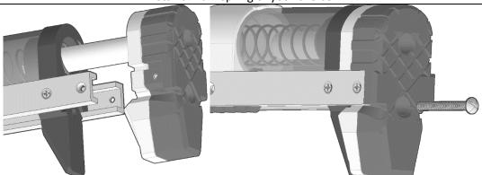
Slide the Butt Assembly into the end of the stock
