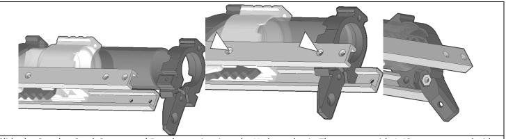
Slide the Coupler, Stock Spacer, and Frontbutt prints into the U-channel pair. Then secure with 4-40 screws on each side.
