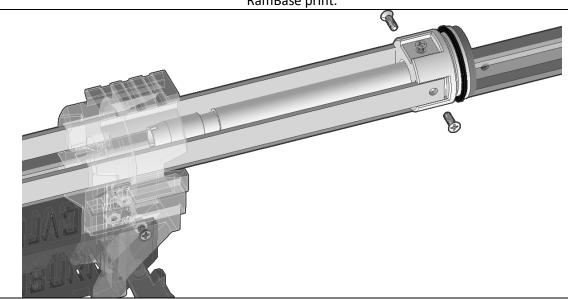
Put the Ramrod Assembly between the bolt arms and secure it with a 4-40 screw driven into it from either side. Set this assembly aside.
