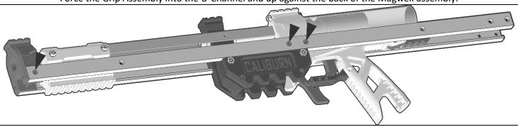
Add the second u-channel as shown to the side of the assembly. Secure it to the magback print with 4-40 screws. Slide the muzzle print into the front end of the u-channel pair and secure it on each side with a 4-40 screw.
