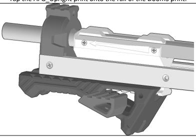
Force the AFGCore into the window of the AFG\_Upright print once the placement lines up with the teeth of the AFGcore print. Force it into place with a hammer until roughly centered.
