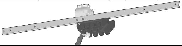
Push one of the U-channels onto the side of the resulting assembly with the two closely-spaced holes towards the rear, and the two further spaced holes towards the front as shown. Line up the hole indicated with the hole in the MagBack print and secure it with a pair of 4-40 screws. If the u-channel doesn't want to be pushed into place you may need to loosen the long 10-32 screw and lower 4-40 screws. Tap it into place with a hammer, then retighten those screws.
