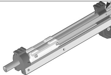
Slide the barrel in through the Muzzle print, DoomS print, and MagFront print until it is flush with the back side of the MagFront print where indicated.
