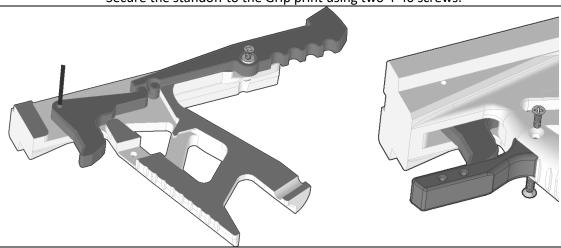
Feed the Trigger print into the slot in the lower front of the Grip print, and wedge the back end of it underneath the front edge of the Sear print. Line up the hole in the Trigger print with the hole in the Grip print and then force a short pin in through both until roughly centered.
