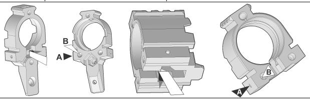
Use a slotted screwdriver to insert and then force a 4-40 hex standoff into the sockets inside the FrontButt print until it bottoms out in it. Drive a 4-40 screw into the hex standoff from the hole in the side of the print until it pulls the standoff to the bottom of the socket.
