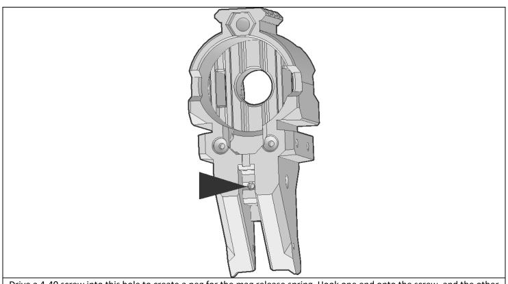
Drive a 4-40 screw into this hole to create a peg for the mag release spring. Hook one end onto the screw, and the other onto the peg on the magrelease print.
