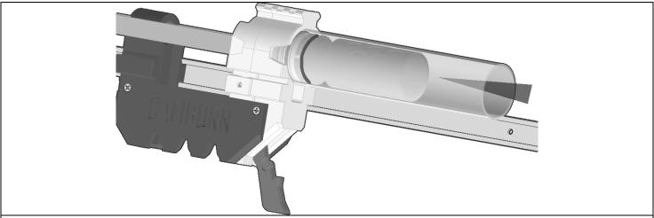
Add an O-ring to the undercut of the PlungerE print, then slide it into the Plunger Tube. Set this assembly aside.
