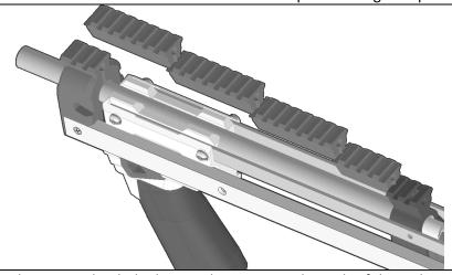
Loosen the screws that hole the muzzle print onto the ends of the u-channel pair. Insert the 3 Rail prints and a RailD print into the gap between the Muzzle and Magfront prints. Orient each so that the positive key in the end of each print faces towards the rear of the blaster.
