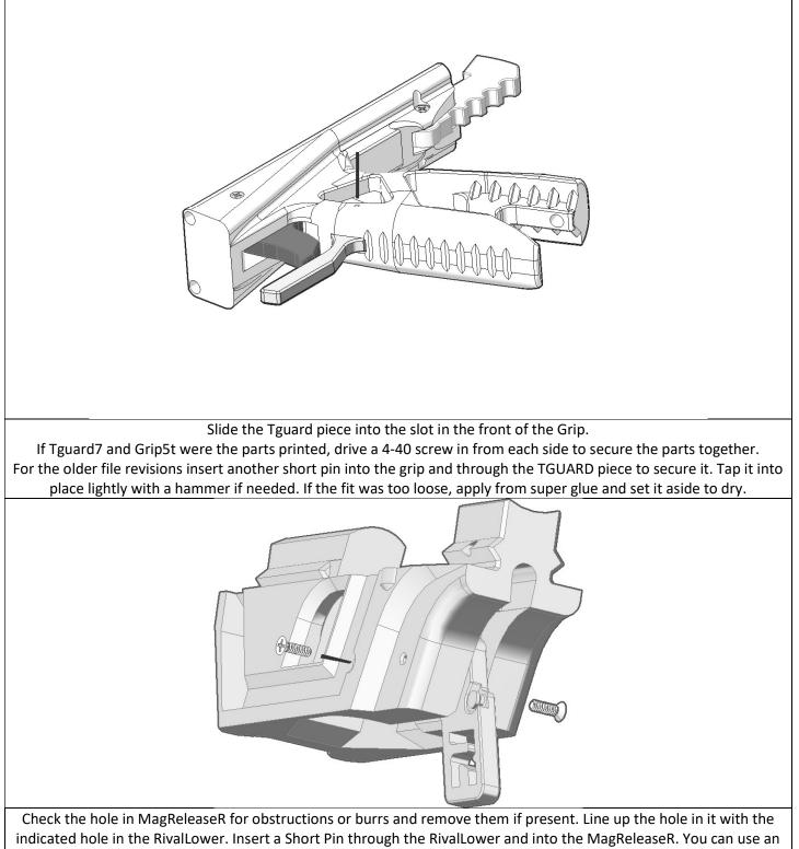
Check the hole in MagReleaseR for obstructions or burrs and remove them if present. Line up the hole in it with the indicated hole in the RivalLower. Insert a Short Pin through the RivalLower and into the MagReleaseR. You can use an extra Short Pin and a Hammer to push it into place. Use a 4-40 screw and a screwdriver to plug the open hole. Repeat for the opposite side of the RivalLower.
