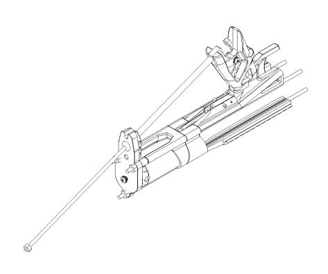
Wedge the 6" spacers inbetween the heel of the Grip and the front angled surface of the Butt. Add a Hex Nut to the very end of the 8" Threaded Rod and then slide it in through the counterbored hole in the Butt. Add a Hex Nut to the opposite end of the 8" Threaded Rod and tigthen.
