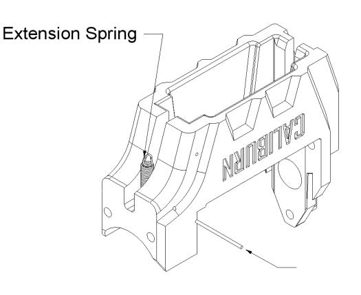
Insert a Pin through the MagWell and through the loop of an Extension Spring. You may need to use a pair of needlenose pliers to get the pin centered. Once it is centered you can push or pry it towards the bottom of the magwell.
