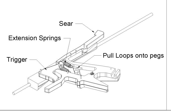
Slide the Sear and Trigger onto their pins. Put the loop of an Extension Springs onto the peg of each. Pull the opposite loop onto the pegs of TGuard2.
