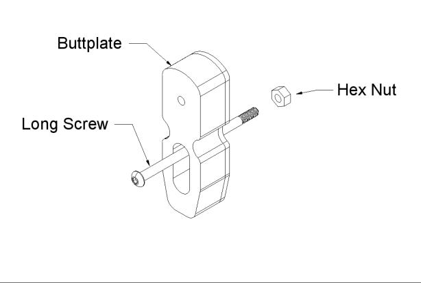
Add the LONG Screw THROUGH THE FOAM and a use a Hex Nut to secure it to the Buttplate (or a Printed Alternative).
