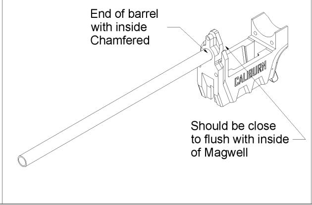
Install the Chamfered side of the Barrel into the Mag Well. You may need to file this hole out with a Round Needle File prior installing the barrel. The inside of the Mag Well can be rested on the edge of a desk or table in order to push the
