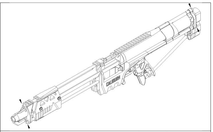
Use six Acorn Nuts to cover the exposed Threaded Rod ends at the front and back of the Blaster.
