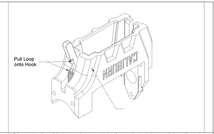
Pull the remaining loop of the Extension Spring onto the hook\peg on the Mag Release. Apply Super Glue to the indicated hole in left left side of the Mag Well or cut a very short section of Dash 123 O-Ring and plug the hole with it. If used, let the glue dry.
