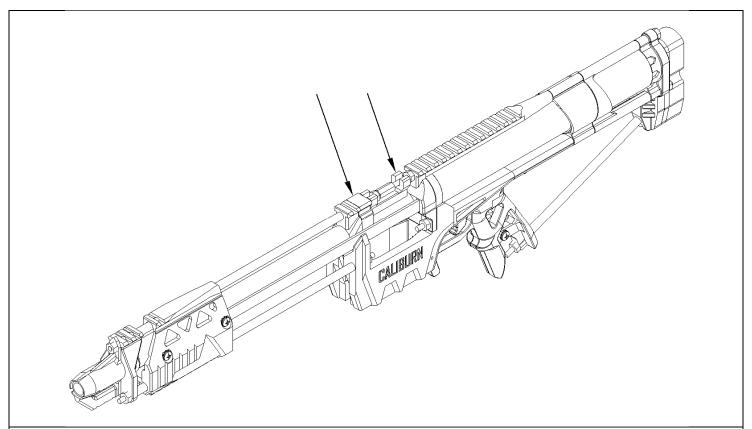
You will need to adjust the positioning of the upper 14" Threaded Rods for this next step, which is why they have not yet been tightened. Slide the Dart Guide onto the front 14" Threaded Rod from the top. Slide the Jam onto both from one side so that the front Hex Nut is behind the tab towards the front of the Blaster. Then rotate the Jam piece until it is oriented vertically.
