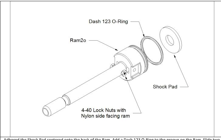
Adhered the Shock Pad centered onto the back of the Ram. Add a Dash 123 O-Ring to the groove on the Ram. Slide two 4-40 Lock Nuts into the slots in the front of the Ram so that their Nylon side is facing the center of the Ram.
