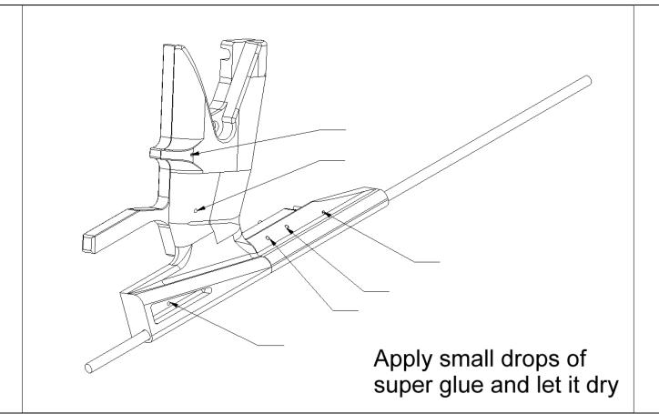
Flip the assembly over and make the ends of the pins flush with the exterior surfaces. Apply a drop of Super Glue to each of the pins and let it dry. This will keep the pins secured to the Right half of the grip assembly.
