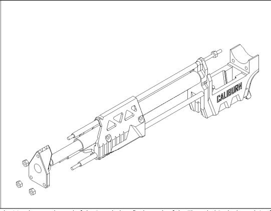
Slide the Muzzle onto the end of the Barrel, then fit the ends of the Threaded Rods through it. If included, slide the Muzzle Brake piece onto the barrel and upper threaded rod. Add three Hex Nuts and tighten the lower two.
