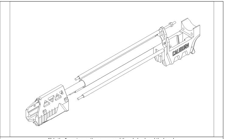
Slide the Foregrip over the now covered threaded rods and the barrel.
