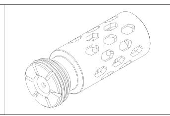
Add a Dash 123 O-Ring to the groove of the Plunger then set aside.
