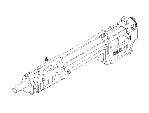
Slide the Foregrip forward. Secure the back half of the Foregrip with two more 1/4" length screws.
