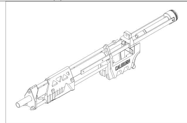
Install the Bolt Assembly by sliding it into the Mag Well from Above. Make sure that the Spreader part is ahead of the lip at the back of the Mag Well.
