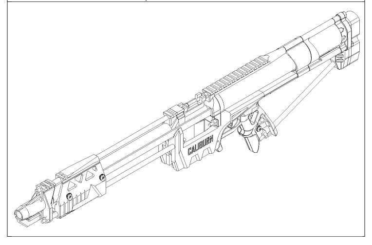
Install a Magazine loaded with darts and cycle the Foregrip back until the catch engages. Slide the foregrip all of the way forwards to chamber the dart in the top of the Magazine. You can load up to four darts into the barrel at a time if desired by cycling the Foregrip back and forth multiple times prior to pulling the Trigger.
