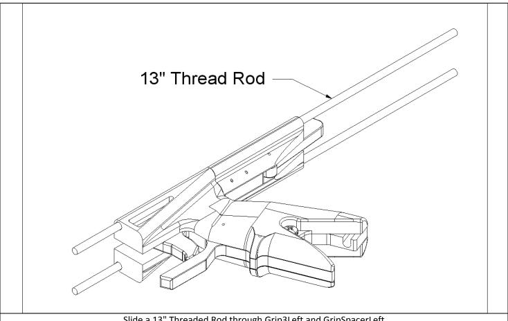
Slide a 13" Threaded Rod through Grip3Left and GripSpacerLeft
