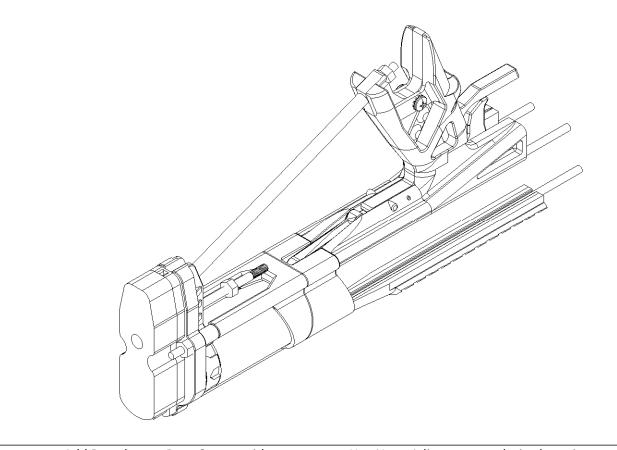
Add Buttplate to Butt. Secure with one or more Hex Nuts. Adjust to your desired spacing.
