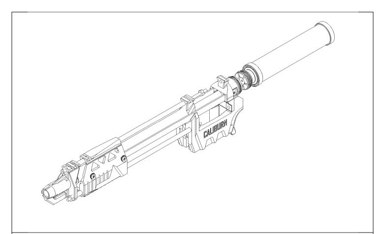
Slide the Plunger backwards into the Lubricated end of the Plunger Tube. Wiggle the Plunger Tube onto the O-Ring at the back end of the Ram Assembly.
