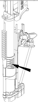
Rest the Buttplate against a chair or table and drop a Main Spring into the Stock. Carefully lower the Plunger Tube and Front Assembly over the Main Spring.
