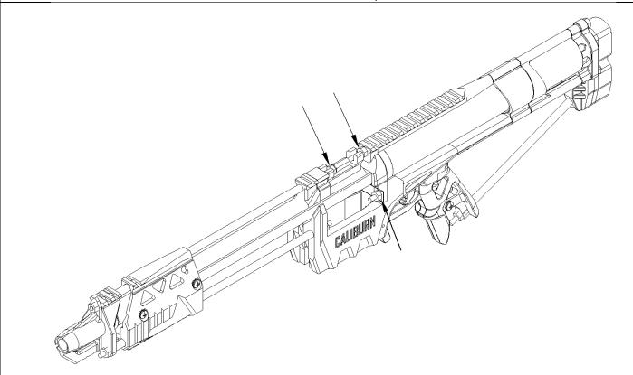
Tighten both of the lower Hex Nuts against Spreader until all of the components of the rear assembly are pulled together firmly. Tighten both Hex Nuts up top. One against the front tab of Jam, the other against Spreader.
