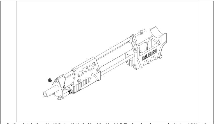
Confirm that the Barrel is still flush with the inside of the Mag Well. The Barrel can be secured using two 1/4" length screws if it has been tapped for them. Otherwise the barrel needs to be glued to the Muzzle using Super Glue or a strong epoxy such as Devon Plastic Weld or Plexus MA310.
