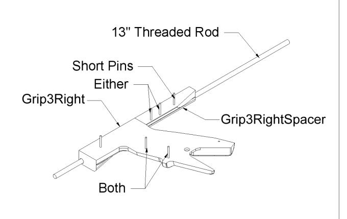
Slide the GripSpacerRight and Grip3Right onto a 13" Threaded Rod. Add Short Pins to most of the small holes as shown.
