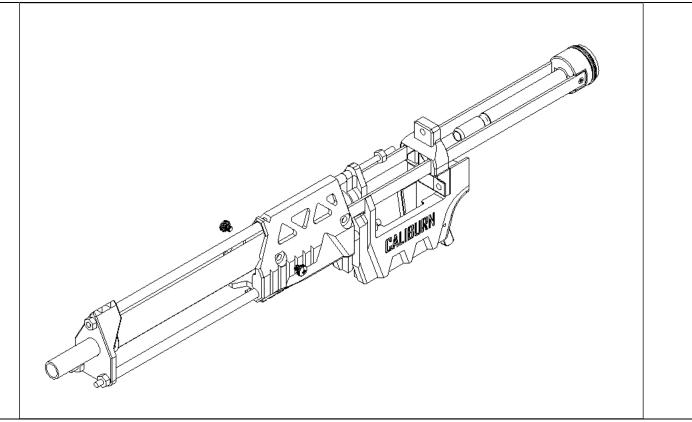
Slide the Foregrip back over the aluminum straps (Bolt Arms) until the threaded holes line up with the holes in the Foregrip. Secure them together at the front pair of holes using two 1/4" length screws. You may need to use a second scredriver or other hand tool to push the aluminum against the inside of the Foregrip so the screw can reach it.
