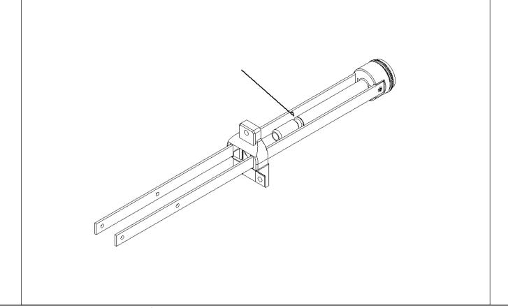
Slide a Spreader over the pair of Bolt Arms. Add an 012 O-ring to the undercut in the Ram. Set this assembly aside temporarily.
