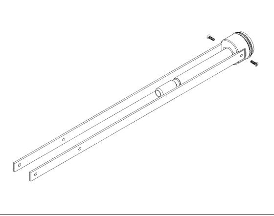
Add two Bolt Arms to the Ram Assembly and secure them with two short 4-40 screws.
