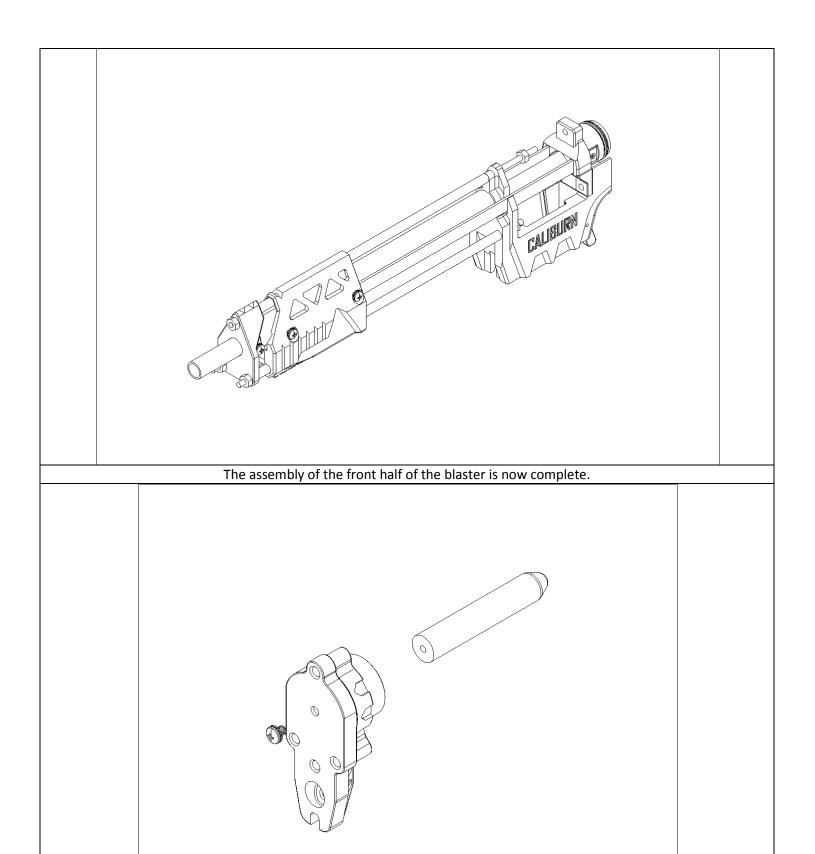
Attach the Stock Core to the Butt piece using a Short Screw.
