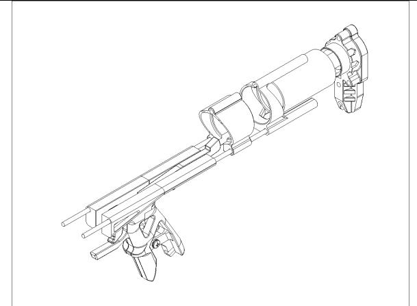
Slide the parts shown onto the 13" Threaded Rods. They include Stock\_Alt2, Ansuzalgiz2, Stock Spacer (clear), and the Butt assembly from earlier.
