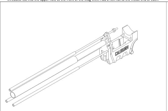
Slide three 11.25 inch length spacers onto the threaded rods. Also slide the Barrel Shroud over the barrel.
