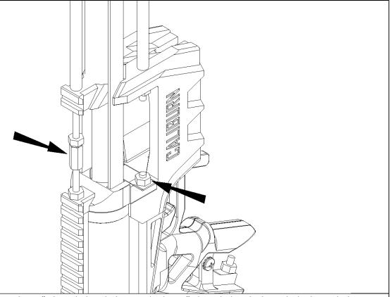
Also add the Coupling Nut to the 14" Threaded Rod, then guide the 13" Threaded Rods through the lower holes in Spreader and add Hex Nuts to those as well. Use the Coupling Nut to connect both 14" Threaded Rods together.
