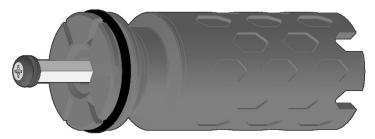
Add a 123 o-ring to the undercut of the PlungerE1 print. Apply and spread some silicone oil onto the rubber grommet and o-ring.
